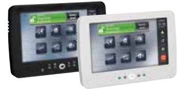
HS2TCHP Hardwired Touchscreen Keypad 7 inch with Prox Support in black and whites
